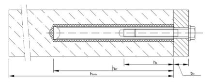
$t_{\text{fix}}$  = thickness of fixture
