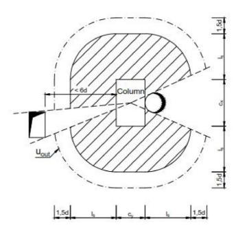
c) Loaded areas (columns) are less than 6d from free edge
