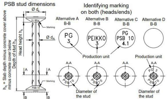
Material: Reinforcing steel with characteristic yield strength f <sub>yk</sub>≥ 500 MPa acc. to EN 1992-1-1 Annex C and data sheet deposited at DIBt
