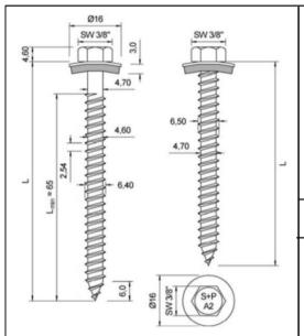
Fastener: Stainless steel A2, A4 or A5 – EN ISO 3506 Washer: Stainless steel A2, A4 or A5 – EN ISO 3506
