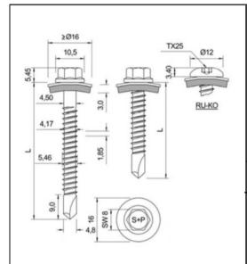
Fastener: Stainless steel A2, A4 or A5 – EN ISO 3506 Washer: Stainless steel A2, A4 or A5 – EN ISO 3506
