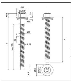
Stainless steel A2, A4 or A5 - EN ISO 3506 Fastener: Stainless steel A2, A4 or A5 - EN ISO 3506 Washer:
