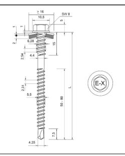
Fastener: stainless Steel (1.4301) - EN 10088 Washer: stainless Steel (1.4301) - EN 10088
