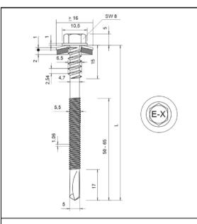
Fastener: stainless Steel (1.4301) - EN 10088 Washer: stainless Steel (1.4301) - EN 10088
