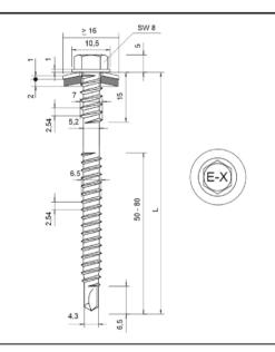
Fastener: stainless Steel (1.4301) - EN 10088 Washer: stainless Steel (1.4301) - EN 10088
