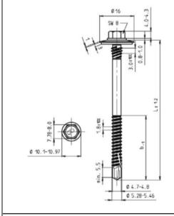
Fastener: Stainless steel A2, A4 or A5 – EN ISO 3506 Washer: Stainless steel A2, A4 or A5 – EN ISO 3506
