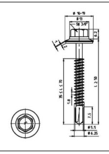
Fastener: Stainless steel A2, A4 or A5 – EN ISO 3506 Washer: Stainless steel A2, A4 or A5 – EN ISO 3506
