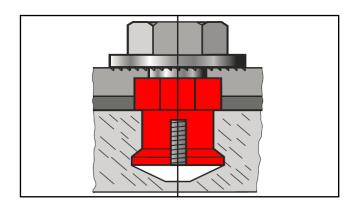
b) Installed undercut anchor
