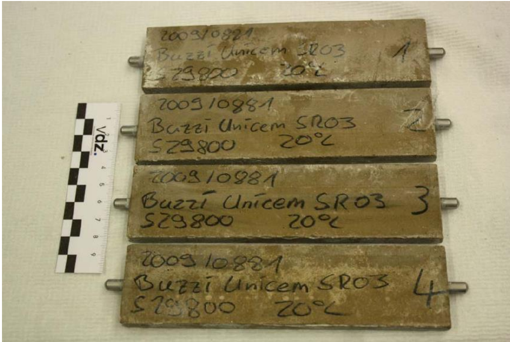
Figure A2.1: Specimens with CSA-based cement "Next Base SR03" after 180 days; Storage: 20 °C in \text{Na}_2\text{O}_4 -solution
