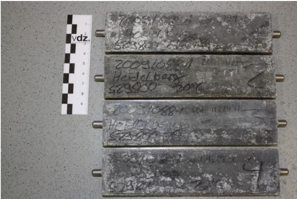
Figure A2.5: Specimens with CEM III/B 42,5 N-LH/SR after 180 days; Storage: 20 °C in Na 2 O 4 -solution
