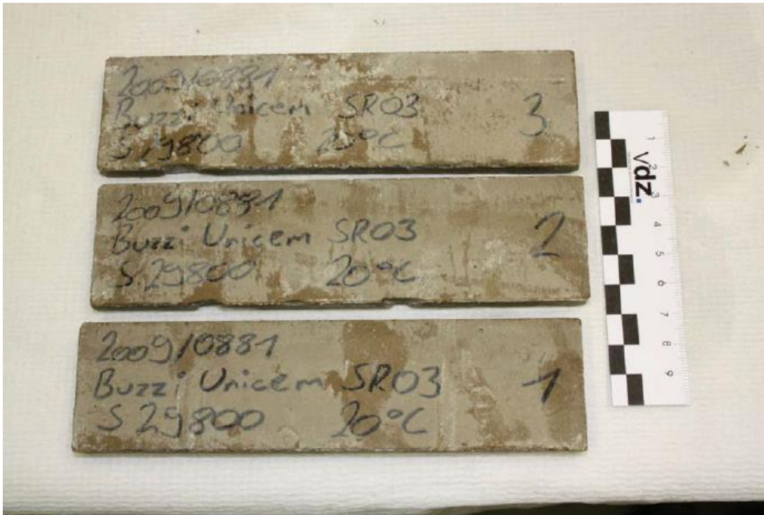
Figure A2.3: Specimens with CSA-based cement "Next Base SR03" after 180 days; Storage: 20 °C in \text{Ca(OH)}_2 -solution
