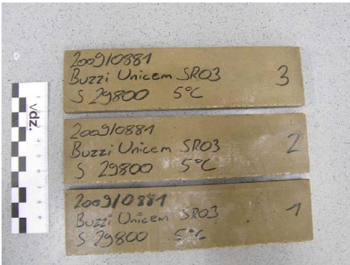
Figure A2.4: Specimens with CSA-based cement "Next Base SR03" after 90 days; Storage: 5 °C in \text{Ca(OH)}_2 -solution
