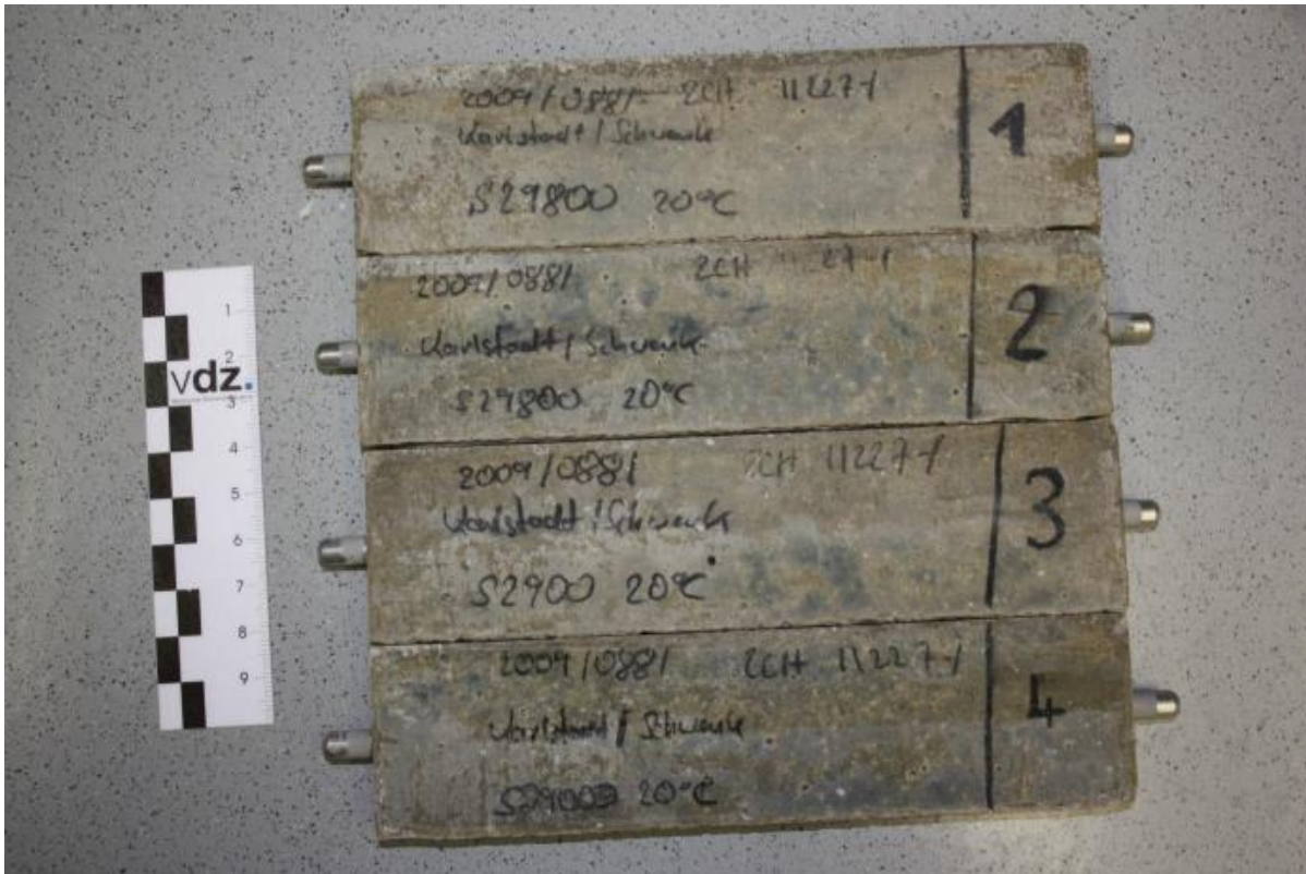
Figure A2.7: Specimens with CEM I 42,5 R-SR3 after 180 days; Storage: 20 °C in Na 2 O 4 -solution
