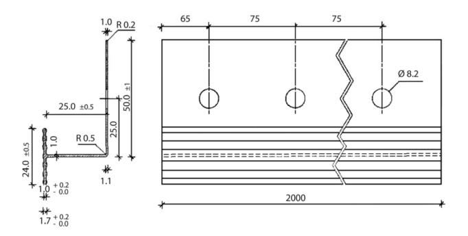
Vertical connection profile – "Verbindungsleiste Alu" (dimensions in millimetres)
