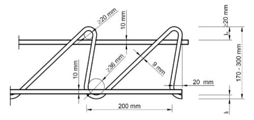
Material: reinforcement steel according EN 1992-1-1, Annex C with a characteristic yield strength of  $f_{yk} = 500 \text{ N/mm}^2$
