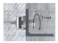
If the anchor channel is embedded below the concrete surface, use washers.
