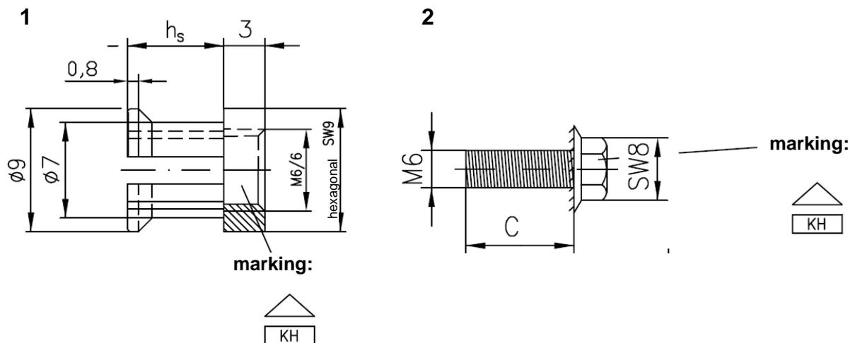
c: The screw length must be adjusted to the respective design
