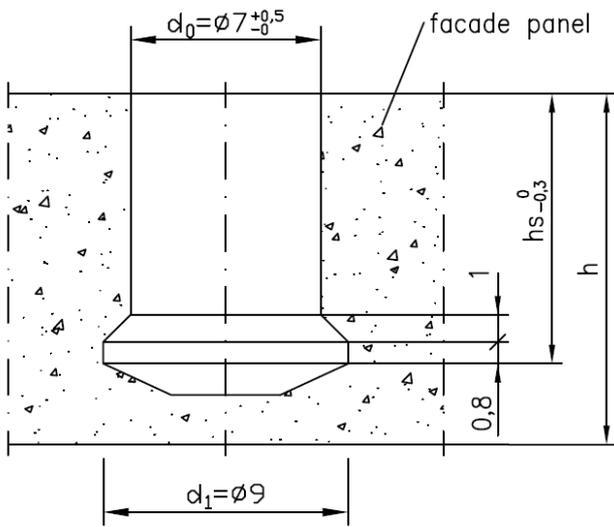
Geometry of the KEIL facade drill
