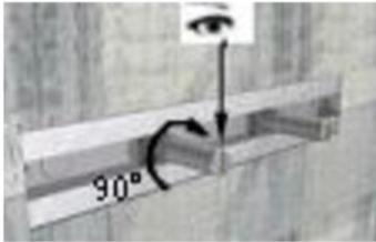
Insert the channel bolt into the slot of the channel. After a 90° turn clockwise, the head of channel bolt locks into the channel.
