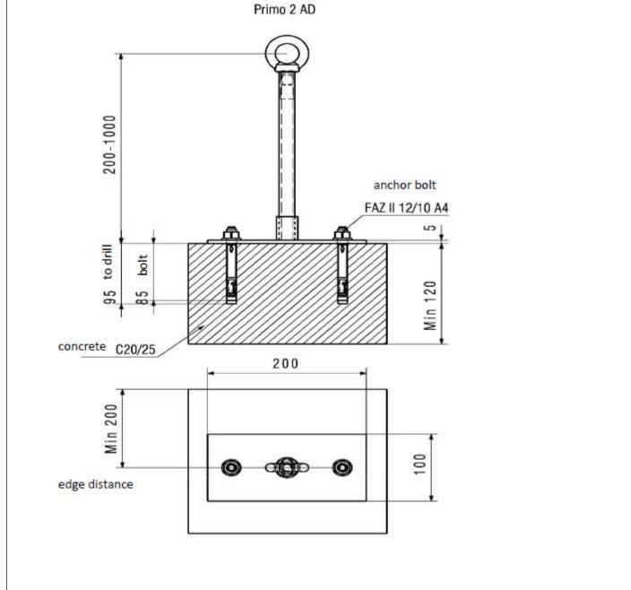
Absturzsicherung Primo 2 AD (Personal Fall Protection System Primo 2 AD) Annex 1 Primo 2 AD for concrete (cracked and uncracked)
