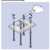
Depending on the further usage anchor bolts have to be fixed at the formwork precisely:
