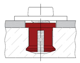
b) Installed undercut anchor
