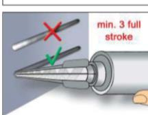
5. Prior to dispensing into the anchor hole, squeeze out separately a minimum of three full strokes and discard non-uniformly mixed adhesive components until the mortar shows a consistent grey colour.
