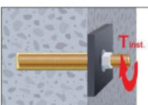
11. After full curing, the add-on part can be installed with up to the max. torque (Table B1 or B3) by using a calibrated torque wrench. It can be optional filled the annular gap between anchor and fixture with mortar. Therefor substitute the washer by the filling washer and connect the mixer reduction nozzle to the tip of the mixer. The annular gap is filled with mortar, when mortar oozes out of the washer.
