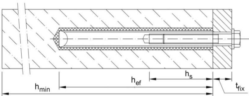
$t_{fix}$  = thickness of fixture
