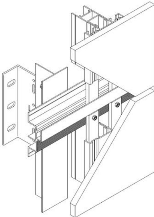
FibreCem-undercut anchor Keil for FibreCem-facade panels
