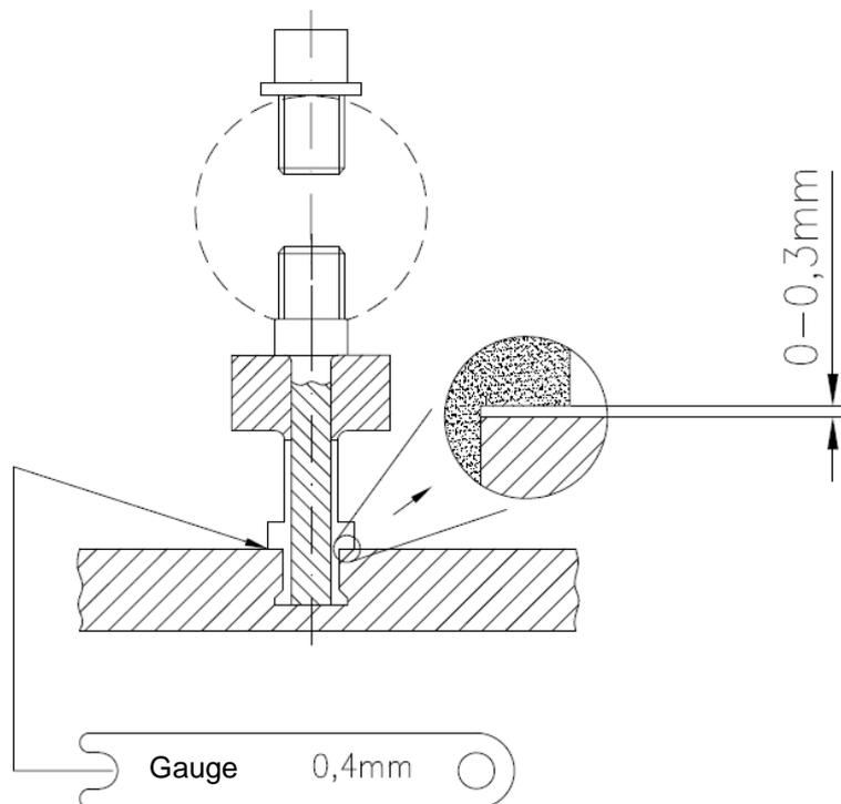
FibreCem-undercut anchor Keil for FibreCem-facade panels
