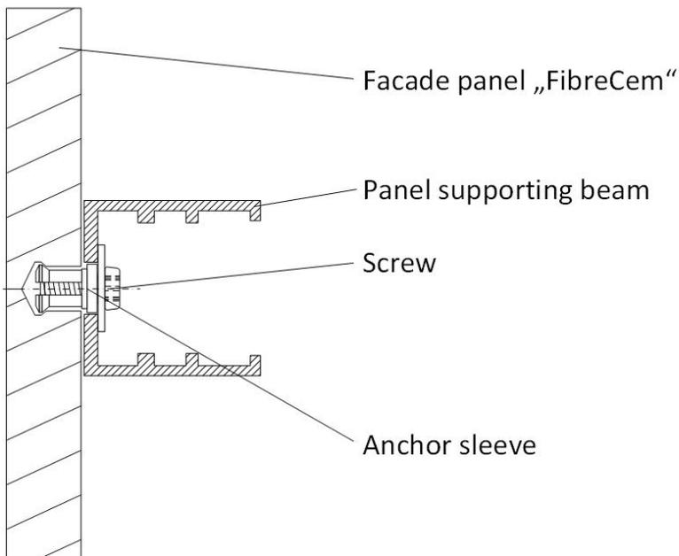
FibreCem-undercut anchor Keil for FibreCem-facade panels
