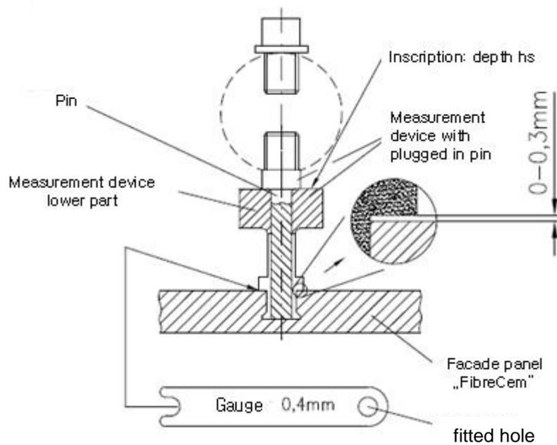
FibreCem-undercut anchor Keil for FibreCem-facade panels
