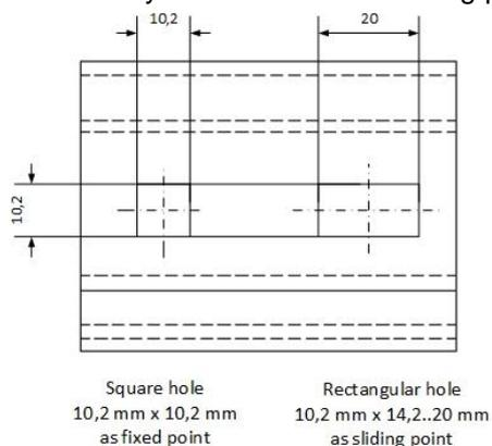
FibreCem-undercut anchor Keil for FibreCem-facade panels
