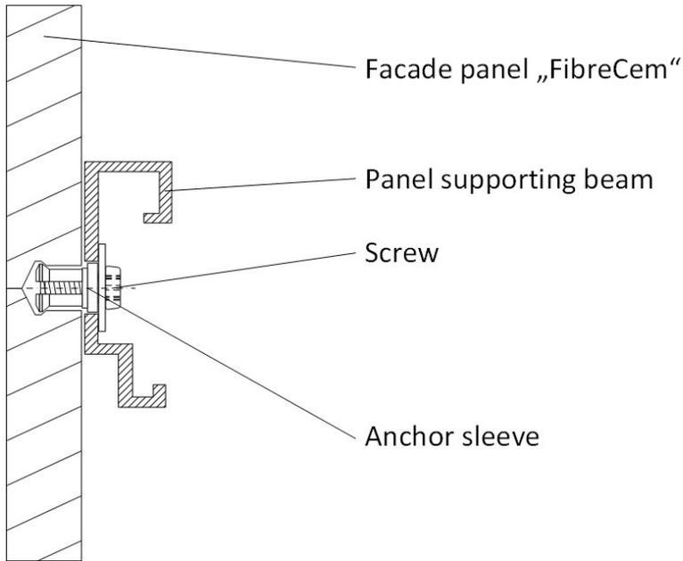
**Fixing example panel supporting beam with facade panel**
