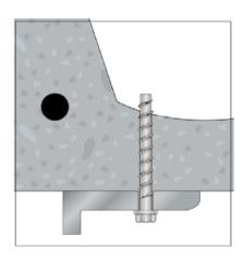
4b. Installation in precast prestressed hollow core slab. Further turning of the anchor is not possible.
