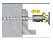
3. Install the anchor with a torque wrench or an Impact Screw Driver using some pressure.
