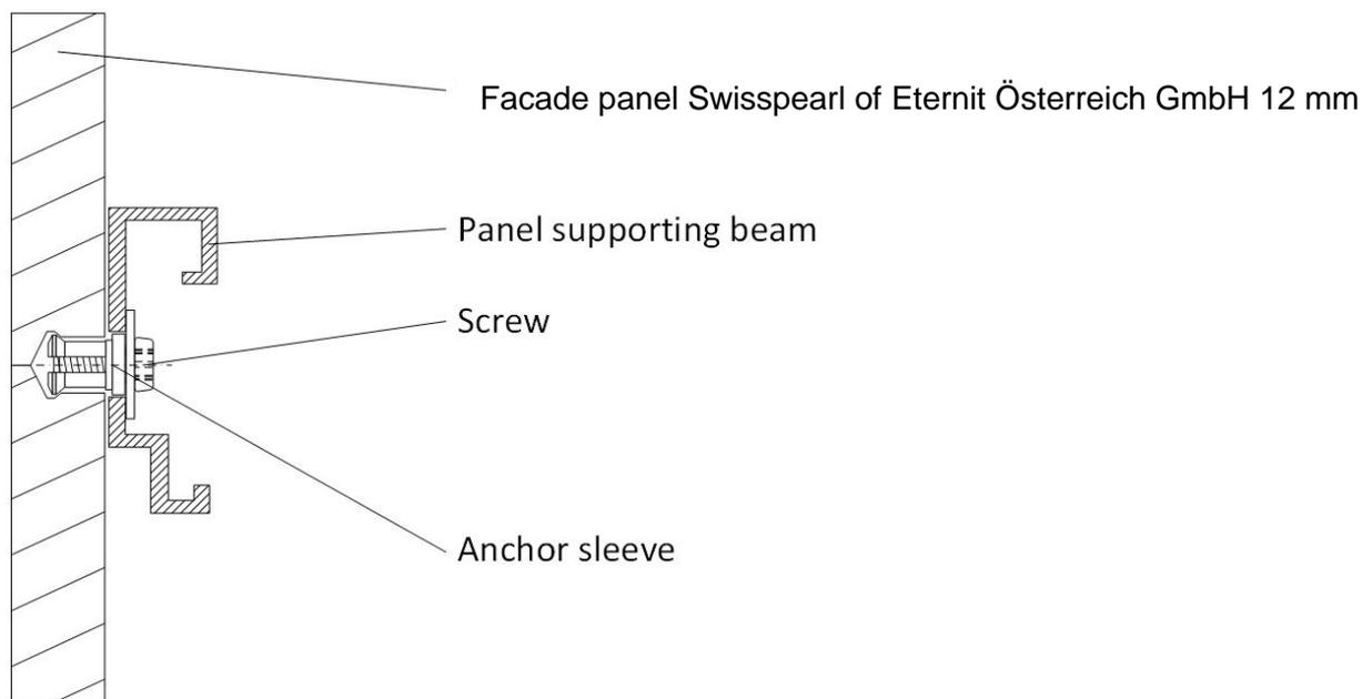
**Fixing example panel supporting beam with facade panel**
