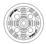
Marking: Identifying Mark (Wkret-Met) Anchor sleeve – LF Anchor size – 10xLa
