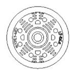
Marking: Identifying Mark (Wkret-Met) Anchor sleeve – LF Anchor size - 8xLa
