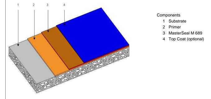
Applicable to the roof waterproofing "MasterSeal M 689"
