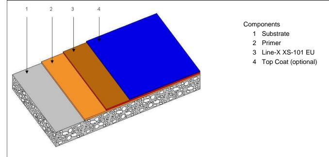
Applicable to the roof waterproofing "Line-X XS-101 EU"
