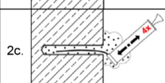
2c. Starting from the bottom or back of the bore hole blow out the hole again a minimum of **four** times.
