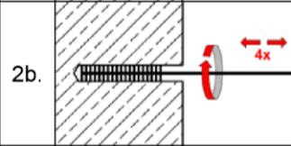
2b. Check brush diameter (Table B4). Brush the hole with an appropriate sized wire brush  $\geq d_{b,min}$  (Table B4) a minimum of **four** times.
