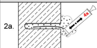
2a. Starting from the bottom or back of the bore hole, blow out the hole with the blow-out pump a minimum of **four** times.
