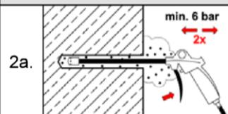
2a. Starting from the bottom or back of the bore hole, blow out the hole with compressed air (min. 6 bar) a minimum of **two** times until return air stream is free of noticeable dust.
