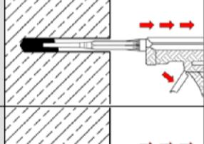
Starting from the bottom or back of the cleaned drill hole fill the hole up to approximately two-thirds with adhesive. Slowly withdraw the static mixing nozzle as the hole fills to avoid air pockets. If the bore hole ground is not reached, an appropriate extension nozzle shall be used.<br>Observe working times given in Table B5.                                                                                                     |
