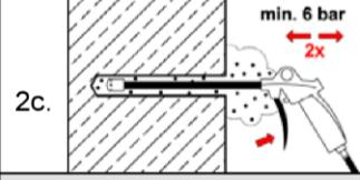
2c. Starting from the bottom or back of the bore hole, blow out the hole with compressed air (min. 6 bar) again a minimum of **two** times until return air stream is free of noticeable dust. If the bore hole ground is not reached, an extension must be used.
