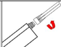
Attach the supplied static-mixing nozzle to the cartridge and load the cartridge into the correct dispensing tool.<br>For every working interruption longer than the recommended working time (Table B5) as well as for new cartridges, a new static-mixer shall be used.                                                                                                                                                                       |
