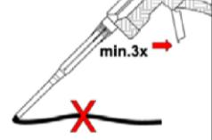
Prior to dispensing into the drill hole, squeeze out separately a minimum of three full strokes and discard non-uniformly mixed adhesive components until the mortar shows a consistent grey colour.                                                                                                                                                                                                                                            |
