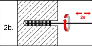
2b. Check brush diameter (Table B4). Brush the hole with an appropriate sized wire brush  $\geq d_{b,min}$  (Table B4) a minimum of **two** times.
