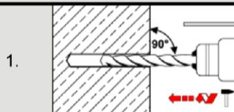
1. Drill with hammer drill or compressed air drill or vacuum drill a hole into the base material to the size required by the selected anchor (Table B1, B2 or B3). In case of aborted drill hole, the drill hole shall be filled with mortar.
