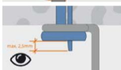
Installed ceiling anchor; control of maximum overlap of shank:
