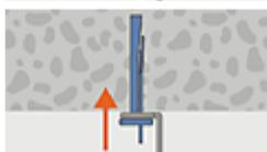
Place the ceiling anchor with the fixture concisely into the hole
