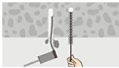
Clean the drill hole from drill dust
