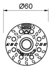
Marking of the anchor sleeve: Anchor type (Combi Fix Plus) Use category A,B,C,D, E
