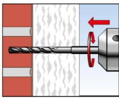
Drill hole by corresponding drilling method.
