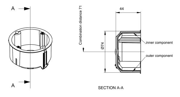
"Geräte-Verbindungsdose/One-gang junction box HWD90", article No 9464-01
