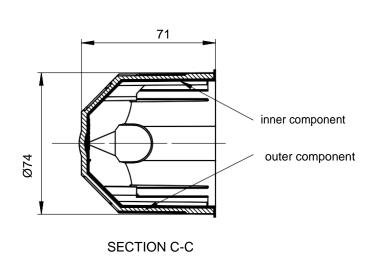
"Brandschutzdose Unterputz/Flush-moulding fire-protection box" article No 1564-01
