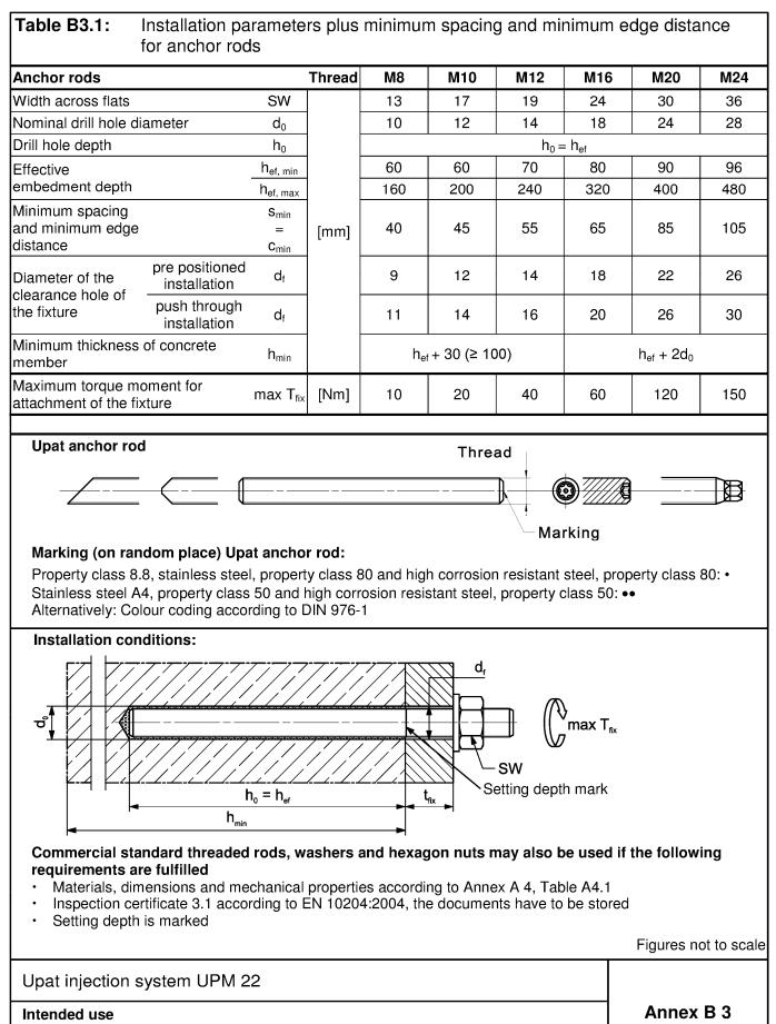
Installation parameters anchor rods
