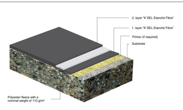
Applicable to the roof waterproofing "K'SEL Etanché Fibre"
