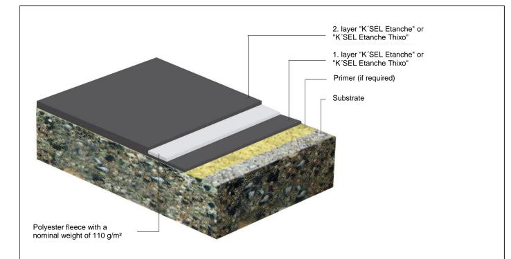
Applicable to the roof waterproofings "K'SEL Etanche" and "K'SEL Etanche Thixo"
