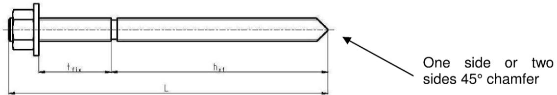
Marking on the CHEMSET™ ANCHOR STUD: letter S, bolt diameter and maximum thickness of the fixture: e.g.: S M10 / 20
