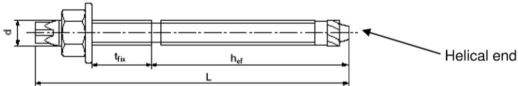
**- CHEMSET™ ANCHOR STUD M8 to M16 with washer and nut (A4)**
