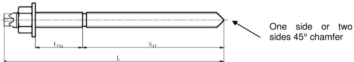
**- CHEMSET™ ANCHOR STUD M20 to M30 with washer and nut (Electroplated / A4)**
