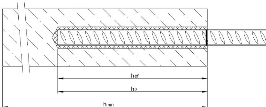
**Installation internal threaded anchor rod IG-M6 up to IG-M20**
