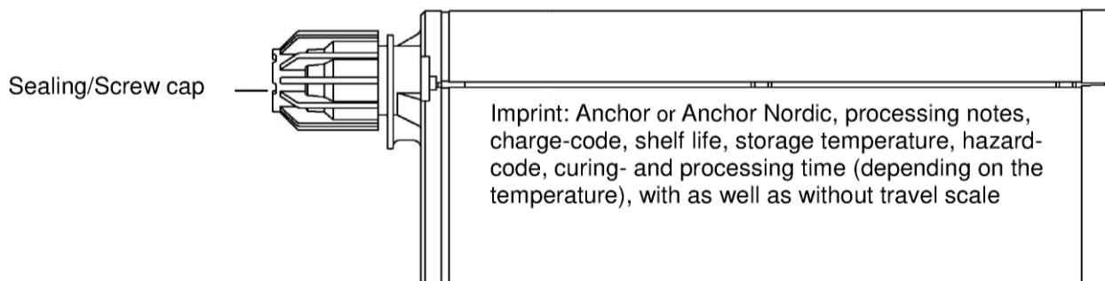
165 ml and 300 ml cartridge (Type: "foil tube")
