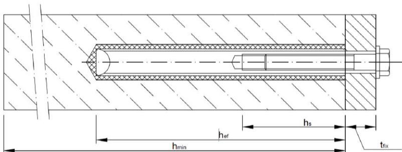
$t_{fix}$  = thickness of fixture
