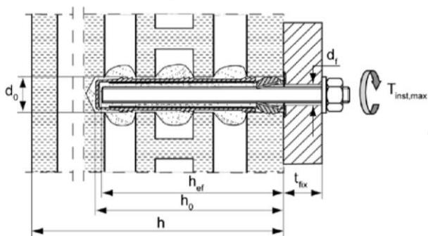
Internal threaded anchor with perforated sleeve
