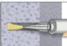
6. Starting from the bottom or back of the cleaned anchor hole, fill the hole up to approximately two-thirds with adhesive. Slowly withdraw the static mixing nozzle as the hole fills to avoid creating air pockets. If the bottom or back of the anchor hole is not reached, an appropriate extension nozzle must be used. Observe the gel-/ working times given in Table B5.
