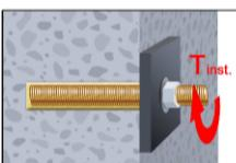
11. After full curing, the add-on part can be installed with up to the max. torque moment (Table B1 or B3) by using a calibrated torque wrench. It can be optional filled the annular gap between anchor and fixture with mortar. Therefor substitute the washer by the filling washer and connect the mixer reduction nozzle to the tip of the mixer. The annular gap is filled with mortar, when mortar oozes out of the washer.
