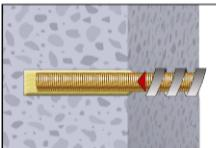
8. Push the anchor rod or reinforcing bar into the anchor hole while turning slightly to ensure positive distribution of the adhesive until the embedment depth is reached.
