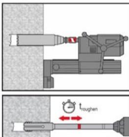
Diamond coring is permissible when suitable diamond core drilling machines and the corresponding core bits are used.
