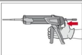
After injection is completed, depressurize the dispenser by pressing the release trigger. This will prevent further adhesive discharge from the mixer.
