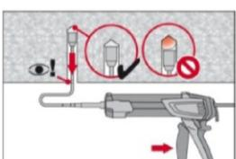
Overhead installation and/or installation with embedment depth  $h_{ef} > 250\text{mm}$ . For overhead installation the injection is only possible with the aid of extensions and piston plugs. Assemble HIT-RE-M mixer, extension(s) and appropriately sized piston plug (see Table B9). Insert piston plug to back of the hole and inject adhesive. During injection the piston plug will be naturally extruded out of the drill hole by the adhesive pressure.
