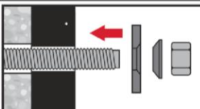
Use Hilti filling set with standard nut. Observe the correct orientation of filling washer and spherical washer.
