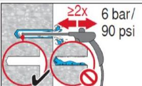
Blow 2 times from the back of the hole (if needed with nozzle extension) over the whole length with oil-free compressed air (min. 6 bar at 6 m<sup>3</sup>/h) until return air stream is free of noticeable dust and water. Remove all water from the borehole until borehole is completely dried before mortar injection. For drill hole diameters  $\geq 32$  mm the compressor has to supply a minimum air flow of 140 m<sup>3</sup>/h.
