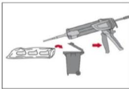
Discard initial adhesive. The foil pack opens automatically as dispensing is initiated. Depending on the size of the foil pack an initial amount of adhesive has to be discarded. Discarded quantities are
