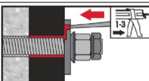
Fill the annular gap between the anchor rod and fixture with 1-3 strokes of Hilti injection mortar HIT-HY 200 A.
