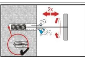
Brush 2 times with the specified brush (see Table B9) by inserting the steel brush Hilti HIT-RB to the back of the hole (if needed with extension) in a twisting motion and removing it.
