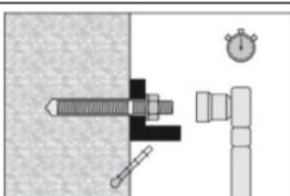
Loading the anchor: After required curing time  $t_{cure}$  (see Table B7 or Table B8) the anchor can be loaded.
