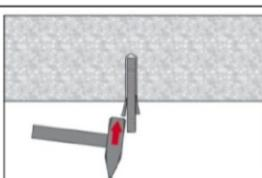
For overhead installation use piston plugs and fix embedded parts with e.g. wedges.
