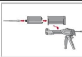
Tightly attach new Hilti mixing nozzle HIT-RE-M to foil pack manifold (snug fit). Do not modify the mixing nozzle.
