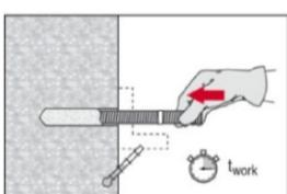
Before use, verify that the element is dry and free of oil and other contaminants. Mark and set element to the required embedment depth until working time  $t_{work}$  has elapsed. The working time  $t_{work}$  is given in Table B7 or Table B8.
