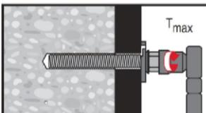
The applied installation torque shall not exceed the values  $T_{\max}$  given in Table B2 to Table B5.
