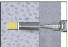
7. Piston plugs and mixer nozzle extensions shall be used according to Table B4 for the following applications:
