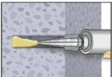
6. Starting from the bottom or back of the cleaned anchor hole, fill the hole up to approximately two-thirds with adhesive. Slowly withdraw the static mixing nozzle as the hole fills to avoid creating air pockets. If the bottom or back of the anchor hole is not reached, an appropriate extension nozzle must be used. Observe the gel-/ working times given in Annex B 6.
