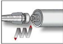
3. Attach the supplied static-mixing nozzle to the cartridge and load the cartridge into the correct dispensing tool. Cut off the foil tube clip before use. For every working interruption longer than the recommended working time (Annex B 6) as well as for new cartridges, a new static-mixer shall be used.
