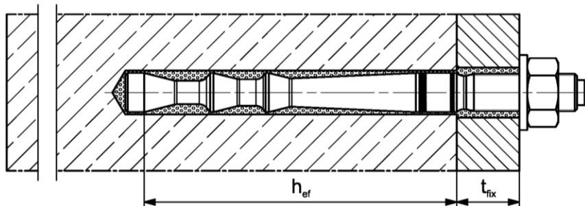
**Pre-positioned or push through installation with subsequently pressed filling disk (annular gap filled with mortar)**
