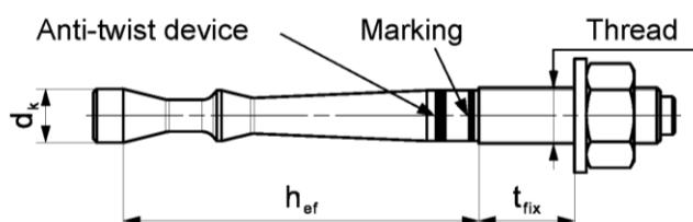
**Marking:** work symbol, size of anchor, setting depth. e.g.: UHB-I M10x75
