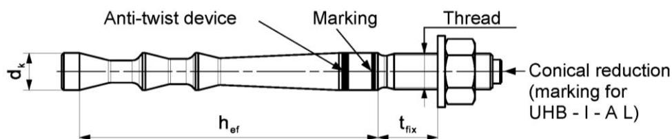
**Marking:** work symbol, size of anchor, setting depth. e.g.: UHB-I M10x95
