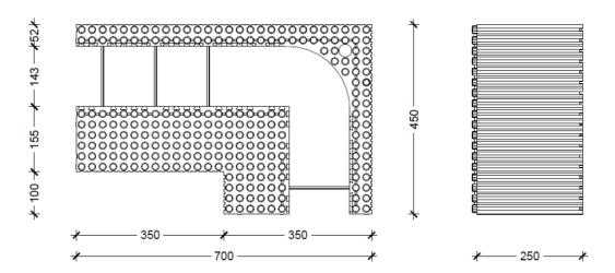
Interior angular elements 45° right/left 747 x 454 x 250 concrete core 143
