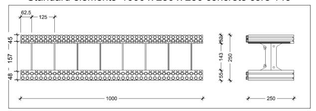
Standard elements with end stops 1000 x 250 x 250 concrete core 143
