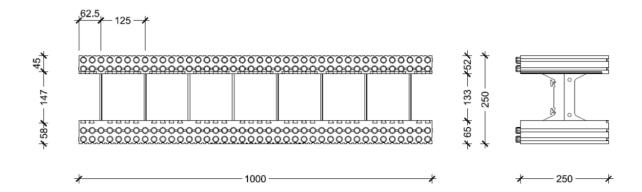
Standard elements with end stops 1000 x 250 x 250 concrete core 133
