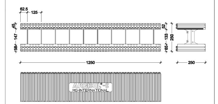
Standard elements with end stops 1250 x 250 x 250 concrete core 133
