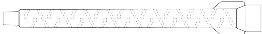
**Threaded rod M8, M10, M12, M16, M20, M24, M27, M30 with washer and hexagon nut**
