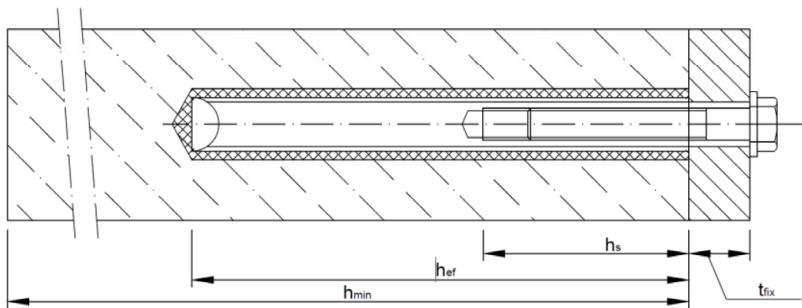
$t_{fix}$  = thickness of fixture
