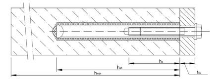
$t_{fix}$  = thickness of fixture
