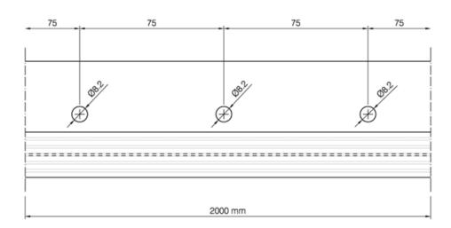
**Vertical connection profile – "Capatect – Verbindungsleiste ALU"** Length: 470 mm
