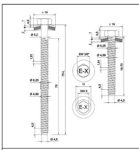
Fastener: stainless Steel (1.4301) - EN 10088 Washer: stainless Steel (1.4301) - EN 10088
