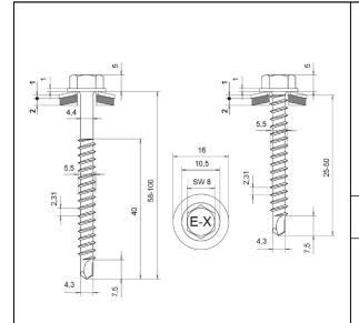
Fastener: stainless Steel (1.4301) - EN 10088 Washer: stainless Steel (1.4301) - EN 10088
