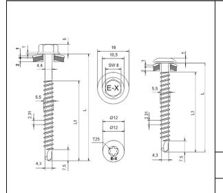
Fastener: stainless Steel (1.4301) - EN 10088 Washer: stainless Steel (1.4301) - EN 10088
