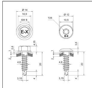
Fastener: stainless Steel (1.4301) - EN 10088 Washer: stainless Steel (1.4301) - EN 10088
