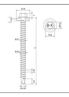
Fastener: stainless Steel (1.4301) - EN 10088 Washer: stainless Steel (1.4301) - EN 10088
