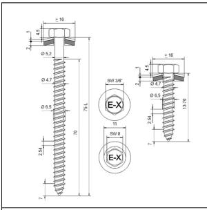
Fastener: stainless Steel (1.4301) - EN 10088 Washer: stainless Steel (1.4301) - EN 10088
