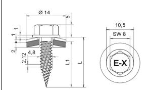
Fastener: stainless Steel (1.4301) - EN 10088 Washer: stainless Steel (1.4301) - EN 10088
