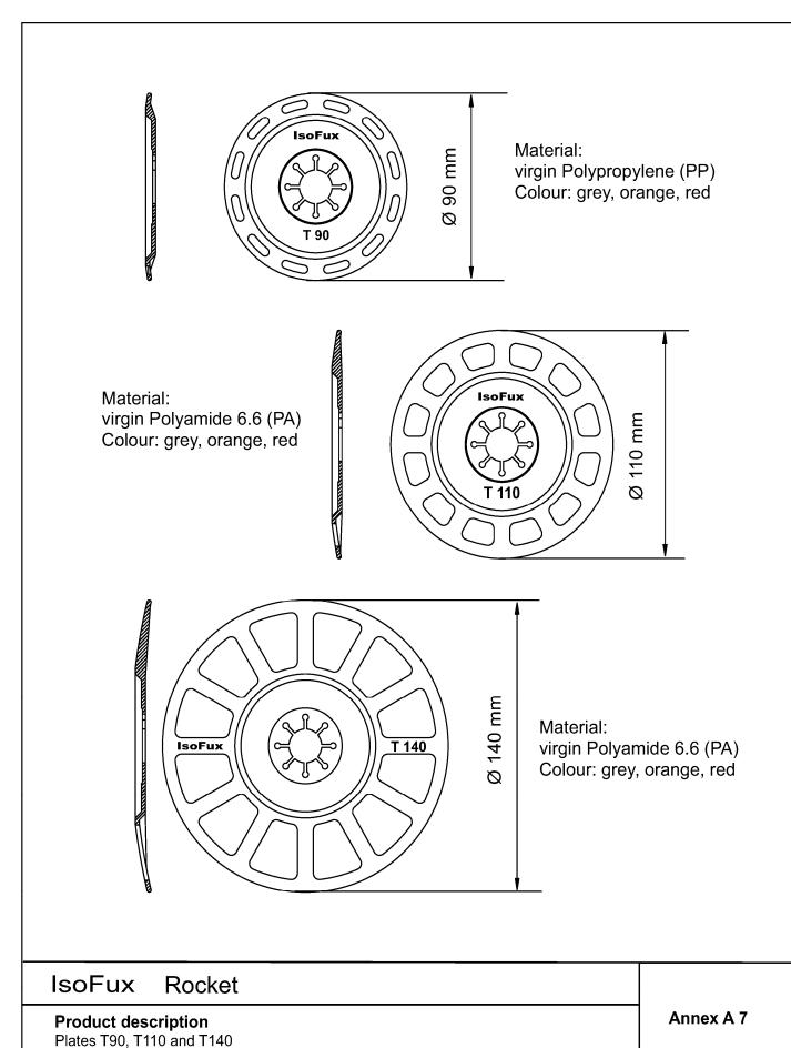
in combination with IsoFux Rocket (for mounting on the surface)
