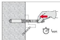
Before use, verify that the element is dry and free of oil and other contaminants. Set element to the required embedment depth before working time  $t_{work}$  has elapsed. The working time  $t_{work}$  is given in Table B4. After setting the element the annular gap between the anchor and the fixture (through-setting) or concrete (pre-setting) has to be filled with mortar.
