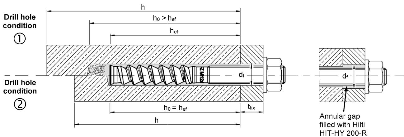
Drill hole condition ① → non-cleaned drill hole
