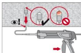
For overhead installation the injection is only possible with the aid of extensions and piston plugs. Assemble HIT-RE-M mixer, extension(s) and appropriately sized piston plug (see Table B5). Insert piston plug to back of the hole and inject adhesive. During injection the piston plug will be naturally extruded out of the drill hole by the adhesive pressure.
