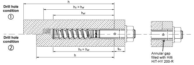
Drill hole condition  $\bigcirc$   $\rightarrow$  non-cleaned drill hole
