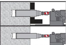
Diamond coring is permissible when suitable diamond core drilling machines and corresponding core bits are used.
