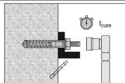
After required curing time  $t_{cure}$  (see Table B4) remove excess mortar. The required installation torque  $T_{inst}$  is given in Table B1. The anchor can be loaded.
