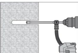
Pre- / Through-setting: Drill hole to the required embedment depth with an appropriately sized Hilti TE-CD or TE-YD hollow drill bit with Hilti vacuum attachment. This drilling system removes the dust and cleans the drill hole during drilling when used in accordance with the user's manual (see Annex A1 – Drill hole condition ②). After drilling is completed, proceed to the "injection preparation" step in the installation instruction.
