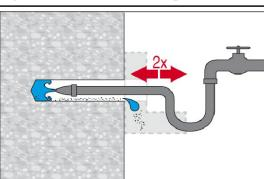
Flush 2 times from the back of the hole over the whole length until water runs clear. Water-line pressure is sufficient.
