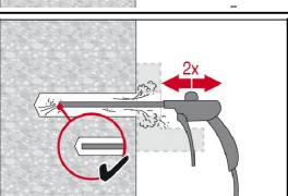
Blow 2 times from the back of the hole (if needed with nozzle extension) with oil-free compressed air (min. 6 bar at 6 m³/h) to evacuate the water.
