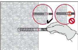
Mark the element and check the setting depth. The element has to fit in the hole until the required embedment depth. If it is not possible to insert the element to the required embedment depth, remove the dust in the drill hole or drill deeper.
