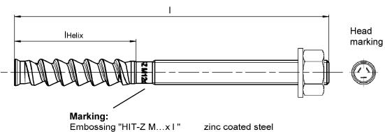
Embossing "HIT-Z-F M...x I" multilayer coating, ZnNi-galvanized Embossing "HIT-Z-R M...x I" stainless steel
