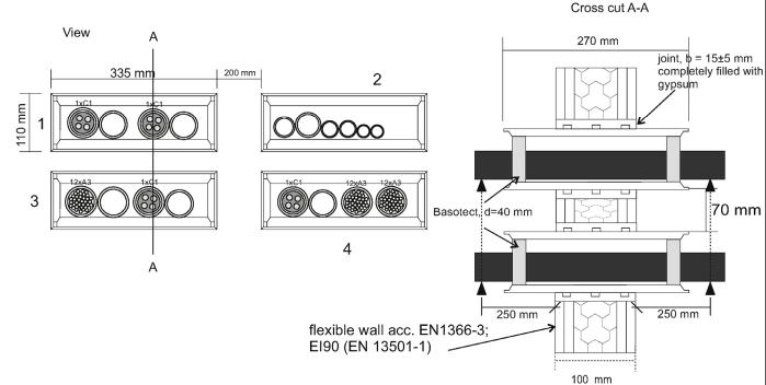
Cable configuration according to EN1366-3:2009-07, all conduits with  $\varnothing$  63 mm
