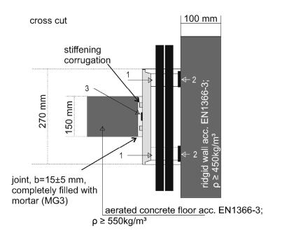
Cable configuration according to EN1366-3:2009-07:
