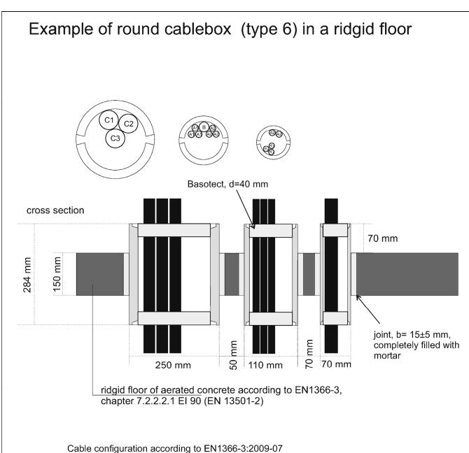
Ø 250 mm Ø 110 mm Ø 70 mm 1xC1-Cable 4x95<sup>2</sup> 1xB-Cable 1x95<sup>2</sup> 3xA1-Cable 5x1,52 1xC2-Cable 4x95<sup>2</sup> 3xA1-Cable 5x1,52 2xA2-Cable 5x1,52 1xC3-Cable 4x95<sup>2</sup> 3xA2-Cable 5x1,52
