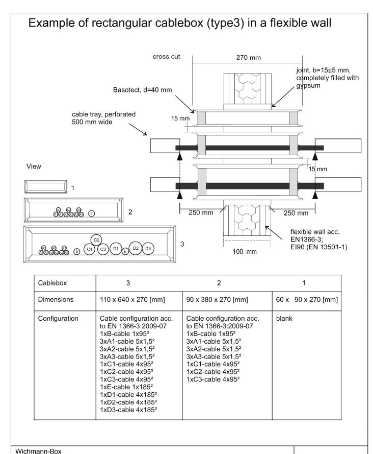
with a fire resistance (integrity and thermal insulation) for more than 90 minutes - Structure of the test specimen; Installation in a flexible wall -
