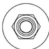
11. Configuration with internal thread and hexagon drive e.g. TSM 6x55 IM M8/10
