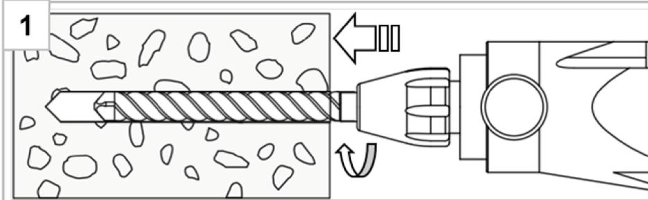
Create hammer drilled or hollow drilled borehole
