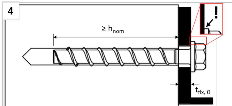
The head must be undamaged and in contact with the fixture
