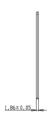
Staple raw wire: ø 1,80±0,03mm Tensile strength  $\geq$  900 N/mm<sup>2</sup> round stainless steel wire WNr. 1.4301 / 1.4401 / 1.4529 or galvanised round wire with zinc thickness  $\geq$  86 g/m<sup>2</sup> Resin coating  $L_H = min. 0.5 L_n$ ;  $\geq 22mm$  Leg length  $L_n = 30.0 - 115.0mm$
