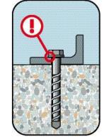
Installation was successful when the head of the anchor is fully supported and in contact to the fixture without damaging it.
