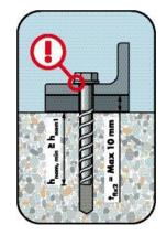
Install the screw again after the adjustment. The total allowed thickness of shims added during the adjustment process is 10mm. The final embedment depth after adjustment process must be equal or larger than h<sub>nom</sub>.
