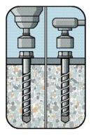
Install the screw by hand or using a impact screw driver. Consider T<sub>imp,max</sub> und T<sub>inst</sub>
