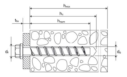
$d_0 = nominal drill bit diameter \\ h_{nom} = nominal anchorage depth \\ h_1 = depth of the drill hole$
